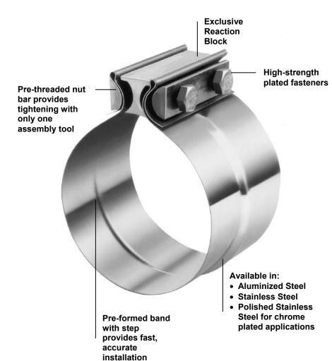
Causes no damaging distortion to pipe or flex. Band is designed for maximum stretch providing tight take-up on pipe/pipe or pipe/flex applications.
