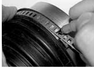
Step 2 Determine the clamp length.
